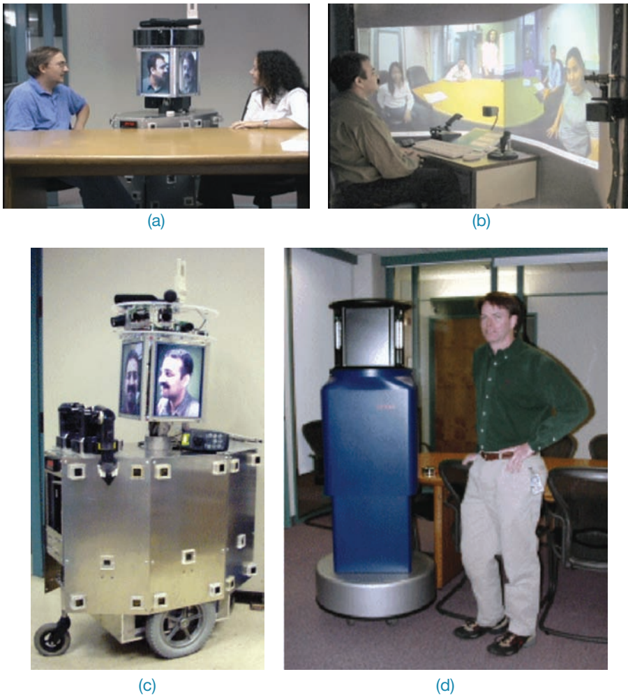
Figure 4.7 BiReality: (a) a surrogate robot at a meeting ‘sitting’ between two physically present people; (b) the remote user’s view of the meeting while controlling the surrogate; (c) an early version of the surrogate on the move; and (d) a second-generation surrogate designed to preserve the height and sitting/standing posture of the user (Jouppi, 2002). See also www.hpl.hp.com/personal/Norman_Jouppi/BiReality240x180v1.3.mov
