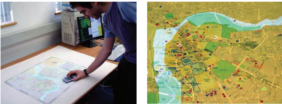
Figure 6.30 An augmented map showing the flooded areas at high water level overlaid on the paper map. The handheld device is used to interact with entities referenced on the map
