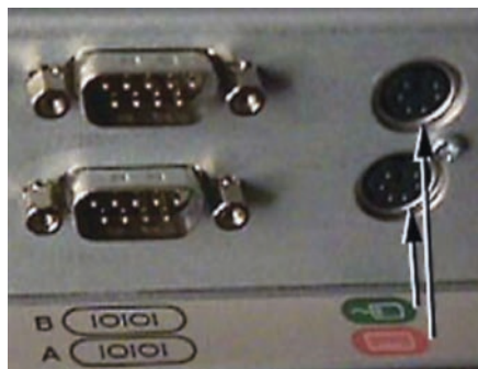
Figure 1.12 Where do you plug in the mouse and keyboard? This figure shows part of the back of a computer. There are two sets of connectors; the two on the right are for a mouse and a keyboard. They look identical and are physically constrained in the same way. How do you know which is which? Do the labels help?
