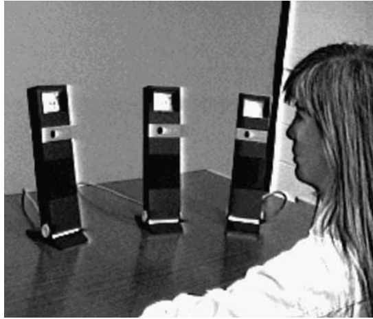
Figure 4.3 The Hydra system: Each hydra unit consists of a camera, monitor, and speaker and is meant to act as a surrogate for a person in a different space. The design is intended to preserve the personal space that people have in face-to-face meetings, simulating where they would sit in the physical space if they were physically present
