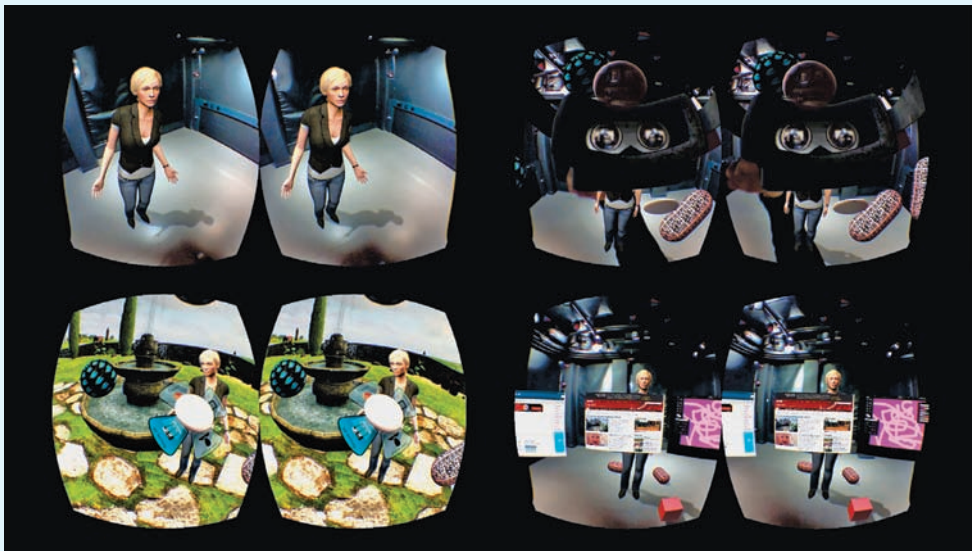
FIGURE 4.10 Oculus Rift: The overlaying of virtual and physical objects to make them appear seamless to the user
